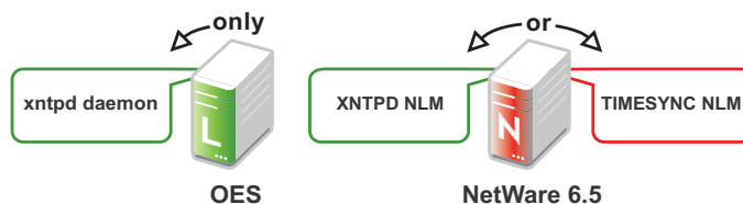
Figure 10-1 Time Synchronization for Linux and NetWare
